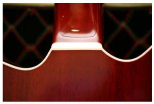
just the original dots, but they're clear and neat. The neck glues precisely into the body with the very tidy binding finishing it off.
